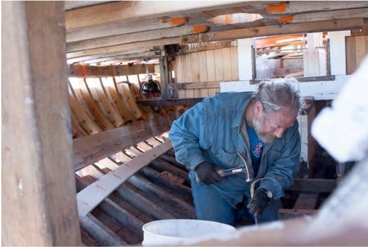
The Woody Guthrie restoration project is continuing to move into the next set of work. As the upper futtocks are now complete, we have been focusing weekend work on prepping for replacement of the lower futtocks. This involved careful marking of positions and removal of the mast step, stem knee, and port and starboard garboards. We are now ready to remove lower futtocks beginning at the bow.
